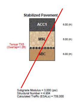
Geogrid option calculated with modified structural coefficient value of 0.17
