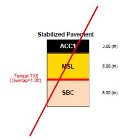
Subgrade Modulus = 3,750 (psi) Structural Number = 3.330 Calculated Traffic (ESALs) = 203,000
