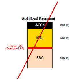
Subgrade Modulus = 3,750 (psi) Structural Number = 2.910 Calculated Traffic (ESALs) = 131,000
