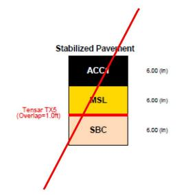
Subgrade Modulus = 3,750 (psi) Structural Number = 4.590 Calculated Traffic (ESALs) = 810,000
