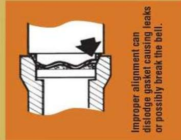
Improper alignment can dislodge gasket causing leaks or possibly break the bell.
