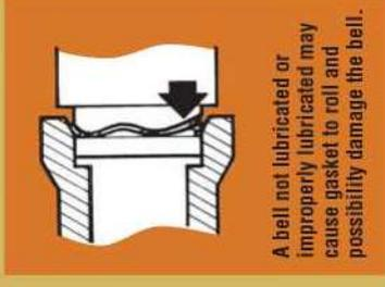
A bell not lubricated or improperly lubricated may cause gasket to roll and possibility damage the bell.
