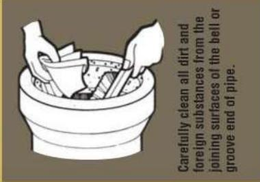
Carefully clean all dirt and foreign substances from the joining surfaces of the bell or groove end of pipe.
