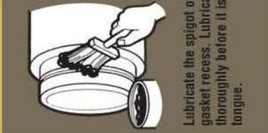
Lubricate the spigot of the pipe, including the gasket recess. Lubricate the o-ring gasket thoroughly before it is placed on the spigot or tongue.
