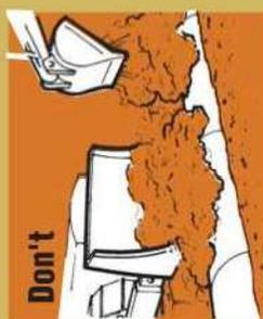
**Don't** Backfill material should be readily compactible and job excavated material and should not contain large stones, boulders, frozen lumps or other objectionable material. Backfill should be placed and compacted in layers as specified.
