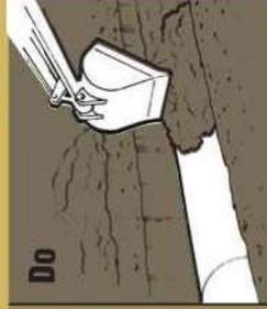
**Do** Backfill material should not be bulldozed into the trench or dropped directly on the pipe. Material should be placed in such a manner so as not to displace or damage the installed pipe.
