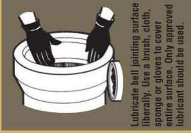
Lubricate bell jointing surface liberally. Use a brush, cloth, sponge or gloves to cover entire surface. Only approved lubricant should be used.
