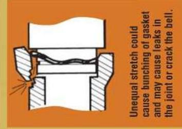
Unequal stretch could cause bunching of gasket and may cause leaks in the joint or crack the bell.
