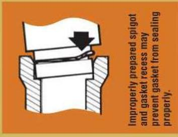
Improperly prepared spigot and gasket recess may prevent gasket from sealing properly.
