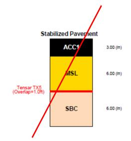
Subgrade Modulus = 6,000 (psi) Structural Number = 3.330 Calculated Traffic (ESALs) = 605,000
