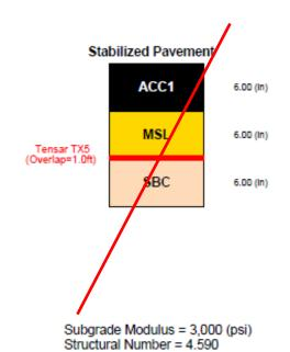
Geogrid option calculated with adjusted structural coefficient value
