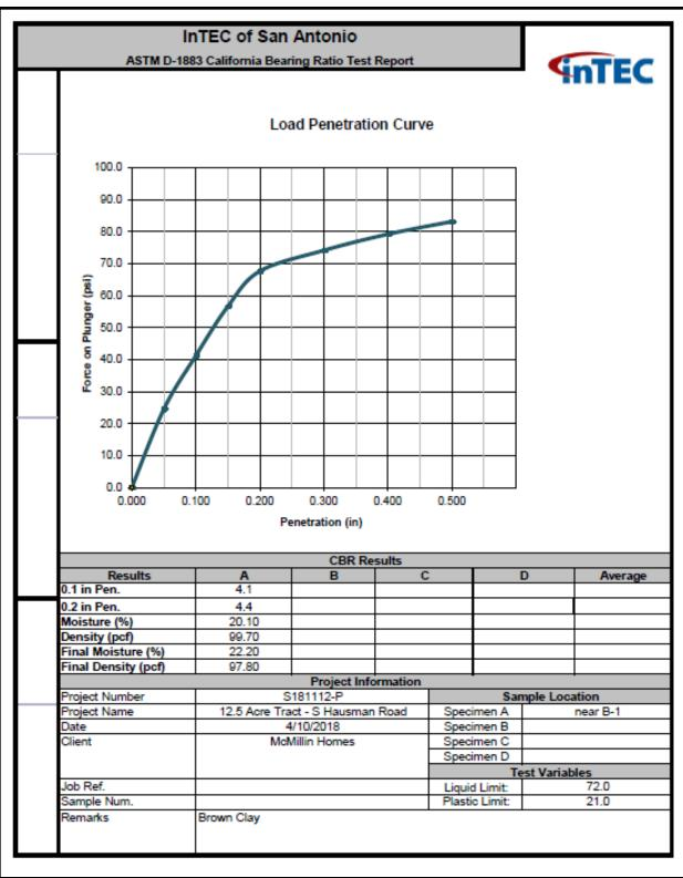
Subsurface Exploration and Pavement Analysis
