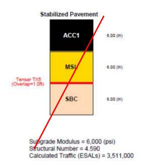
Geogrid option calculated with adjusted structural coefficient value
