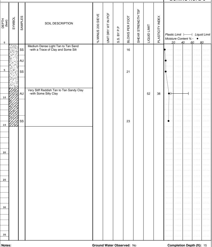
S.S by P.P - Shear Strength in TSF by Hand Penetrometer
