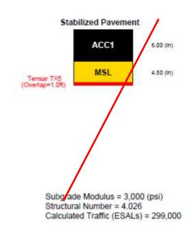
Geogrid option calculated with adjusted structural coefficient value (0.17)
