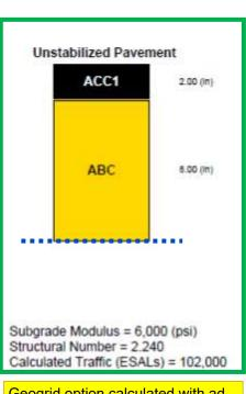
Geogrid option calculated with adjusted structural coefficient value
