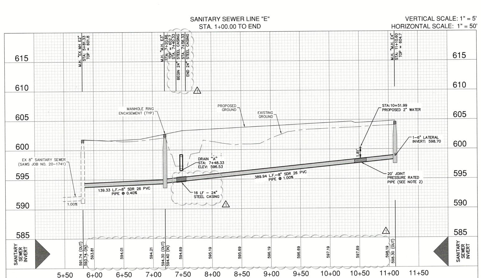
$\triangle$ FINISHED GROUND/PAVEMENT REFERENCE SAWS SPEC ITEM 812 (TOP OF GRADE) ALLALAN P PROPOSED WATER LINE -WHERE SEWER PIPE CROSSES A WATER LINE, THE SEWER SEPARATION DISTANCE AND SHALL BE 160 PSI AND MEET PROTECTION REQUIREMENTS THE REQUIREMENTS OF ASTM TO COMPLY WITH 30 TAC D2241 WITH ONE 20' JOINT 217.53(d) AND 290.44(e) CENTERED AT THE WATER CROSSING PROPOSED SANITARY SEWER LINE TYPICAL SANITARY SEWER/WATER CROSSING DETAIL
