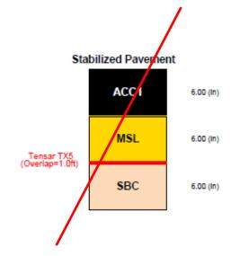
Subgrade Modulus = 3,750 (psi) Structural Number = 4.590 Calculated Traffic (ESALs) = 1,894,000
