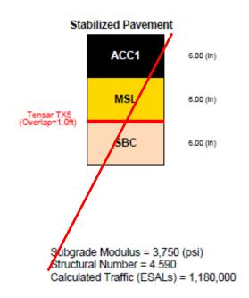
Geogrid option calculated with adjusted structural coefficient value of 0.17
