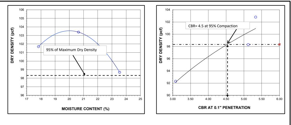
Sample:CBR Sample No. 2Proctor Test Method: Standard Proctor (ASTM D-698)CBR Test Method: California Bearing Ration (ASTM D-1883)Material:FAT CLAY (CH), Very Dark Brown
