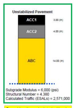
Geogrid option calculated with adjusted structural coefficient value
