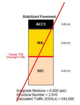
Geogrid option calculated with adjusted structural coefficient value
