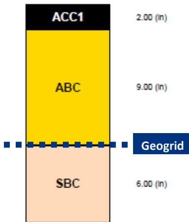
Geogrid option calculated with adjusted structural coefficient value (0.17)
