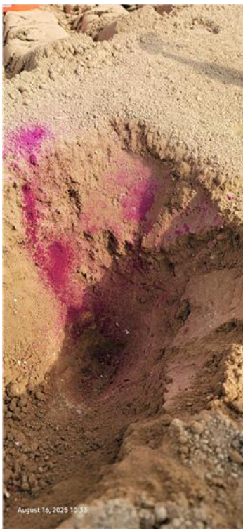
Granite Garden STA 11+00 Phenolphthalein Test
