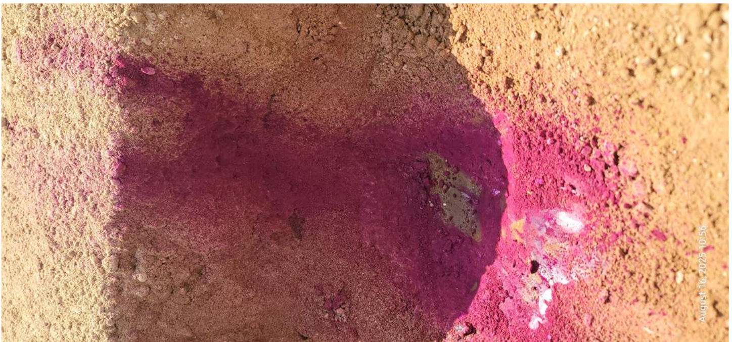
Chalk Cave STA 3+50 Phenolphthalein Test Closeup
