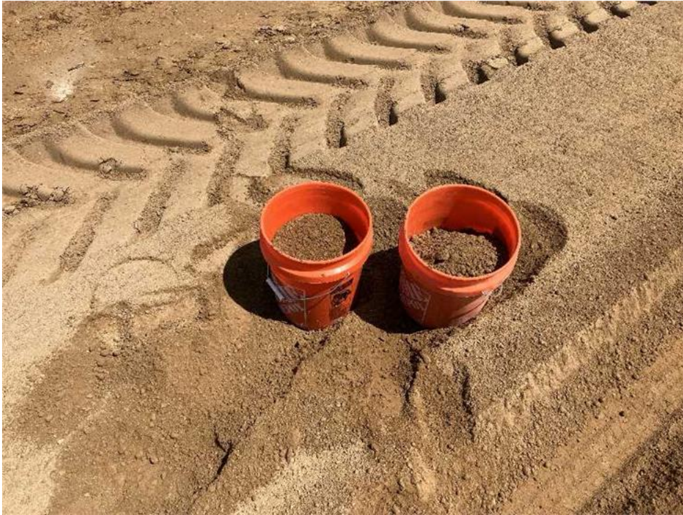
Lime treated subgrade proctor collection at Azzurro Stone near station 5+00
