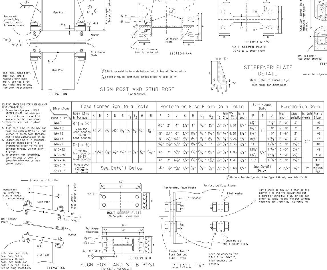
Typ. Weld=Flg. thickness-1/16
