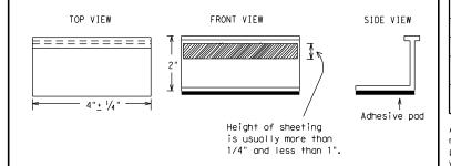
STAPLES OR NAILS SHALL NOT BE USED TO SECURE TEMPORARY FLEXIBLE-REFLECTIVE ROADWAY MARKER TABS TO THE PAVEMENT SURFACE
