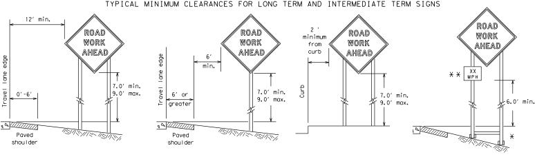
\* When placing skid supports on unlevel ground, the leg post lengths must be adjusted so the sign appears straight and plumb.
