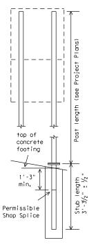
The weight of one S4x7.7 post is equal to 112.2 lbs. plus 7.7 lbs./ft x (post length in feet minus 10 ft). The weight of 112.2 lbs. includes 10 feet of post length, post foundation stub, related connection plates, friction fuse plate, and all high strength bolts, nuts and
