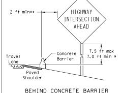
\*\*Sign clearance based on distance required for proper guard rail or concrete barrier performance.
