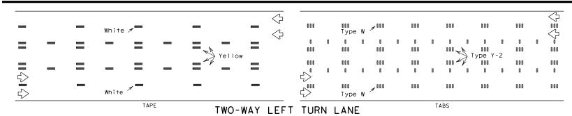
Removable Raised Short Term Pavement Pavement | Marker Markina (Tape)
