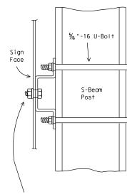
Galvanized steel or aluminum self-locking hex. head nut. 3/8 " - 16 x 3/4 " hex. head bolt for sheet metal. 3/8 " -  $16 \times 1$  1/4 " hex. head bolt for plywood. 3/8 " galvanized medium washer.
