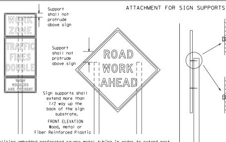
Splicing embedded perforated square metal tubing in order to extend post height will only be allowed when the splice is made using four bolts, two above and two below the spice point. Splice must be located entirely behind the sign substrate, not near the base of the support. Splice insert lengths should be at least 5 times nominal post size, centered on the splice and of at least the same gauge material.
