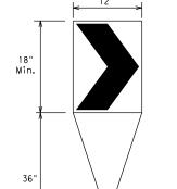
Fixed Base w/ Approved Adhesive (Driveable Base, or Flexible Support can be used)
