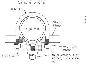
Bolts used to mount sign panels to the clamp are 5/16-18 UNC galvanized square head with nut, nylon washer, flat washer and lock washer. The bolt length is 1 inch for aluminum.
