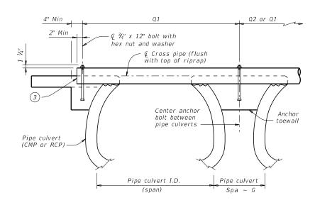
SHOWING CROSS PIPE WITH BOLTED ANCHOR
