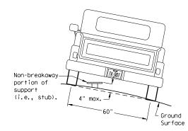
To avoid vehicle undercarriage snagging, any substantial remains of a breakaway support. when it is broken away, should not project more than 4 inches above a 60-inch chord (i.e., typical space between wheel paths).
