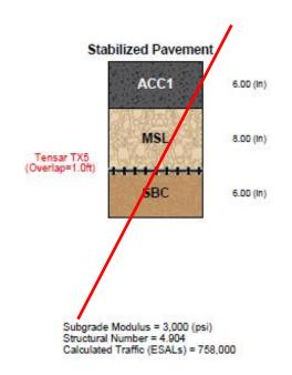
Geogrid option calculated with modified structural coefficient value of 0.17
