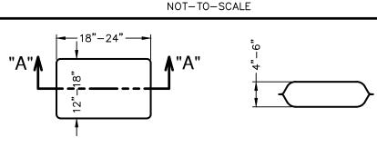
**PLAN VIEW** SECTION "A-A' THE FILTER BAG MATERIAL SHALL BE MADE OF POLYPROPYLENE, POLYETHYLENE OR POLYAMIDE WOVEN FABRIC, MIN. UNIT WEIGHT OF 4
