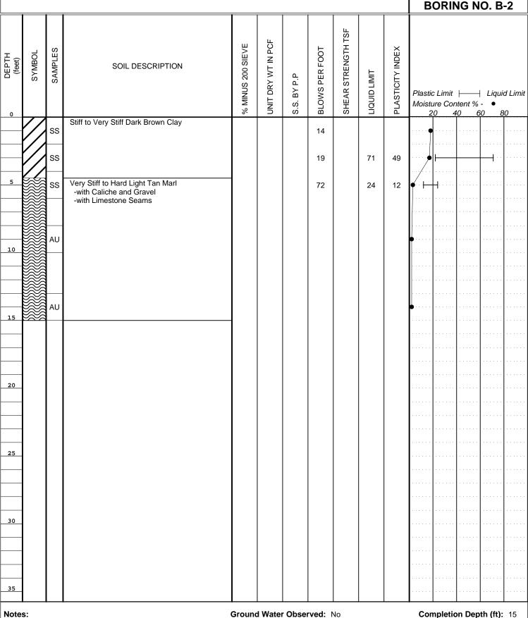
S.S by P.P - Shear Strength in TSF by Hand Penetrometer S.S. - Split Spoon Sample S.T. - Shelby Tube Sample **HA - Hand Auger** AU - Auger Sample
