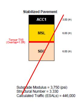
Geogrid option calculated with adjusted structural coefficient value of 0.17
