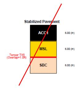
Subgrade Modulus = 3,750 (psi) Structural Number = 4.590 Calculated Traffic (ESALs) = 1,894,000
