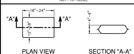
THE FILTER BAG MATERIAL SHALL BE MADE OF POLYPROPYLENE. POLYETHYLENE OR POLYAMIDE WOVEN FABRIC, MIN. UNIT WEIGHT OF 4 OUNCES/SY, HAVE A MULLEN BURST STRENGTH EXCEEDING 300 PSI AND ULTRAVIOLET STABILITY EXCEEDING 70%.
