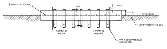
COMPACTED TXDOT GRADE 4, TYPE A, FLEXIBLE BASE MATERIAL, OR OTHER APPROVED MATERIAL FROM BOTTOM OF TRENCH TO BOTTOM OF PAD.
