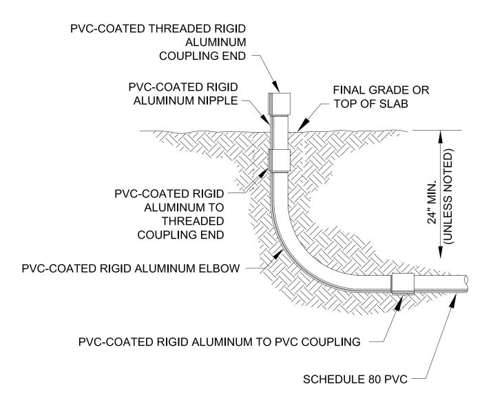
D DUCTBANK TRANSITION DETAIL (TYPICAL)
