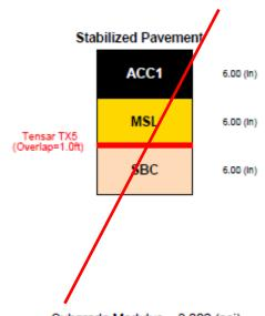
Subgrade Modulus = 3,000 (psi) Structural Number = 4.590 Calculated Traffic (ESALs) = 703,000
