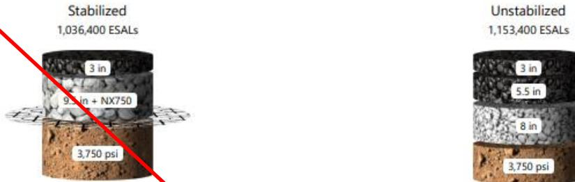
Total HMA thickness should be within the same range on both pavement sections for accurate comparison: 2-3 in | 3-6 in | 6-14 in
