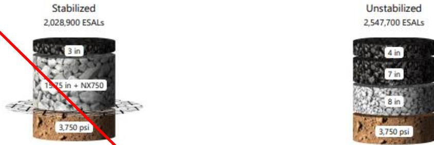
Total HMA thickness should be within the same range on both pavement sections for accurate comparison: 2-3 in | 3-6 in | 6-14 in
